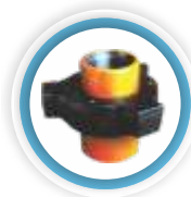
Fig. 602 Black Nut Orange Subs A replaceable lip-type seal ring minimizes fluid flow turbulence and gives pressure seal for air. Water, oil, gas and mud service to 6,000 psi NSCWP*.
