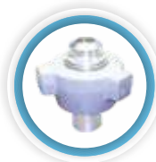
Fig. 602 Black Nut Orange Subs A replaceable lip-type seal ring minimizes fluid flow turbulence and gives pressure seal for air. Water, oil, gas and mud service to 6,000 psi NSCWP*.
